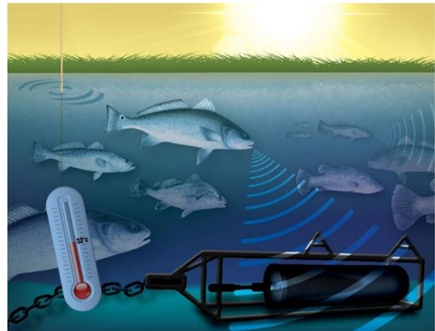
Fig. 7. Long-term acoustic recorders (black instrument in figure) estimate spawning timelines by detecting fish calls associated with courtship. (Monczak et al. 2017. *Marine Ecology Progress Series* 581:1-19. Feature Article)
